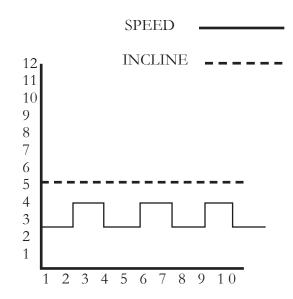
The **Cardio Program** is designed to vary the treadmill Speed, while maintaining a constant Elevation.
